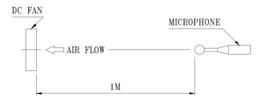
NOISE IS MEASURED AT RATED VOLTAGE IN FREE AIR IN ANECHOIC CHAMBER WITH B & K SOUND LEVEL METER WITH MICROPHONE AT A DISTANCE OF ONE METER FROM THE FAN INTAKE.
