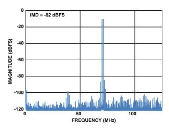
FIGURE 23. TWO-TONE SPECTRUM (F1 = 70MHz, F2 = 71MHz AT -7dBFS) (250MSPS)
