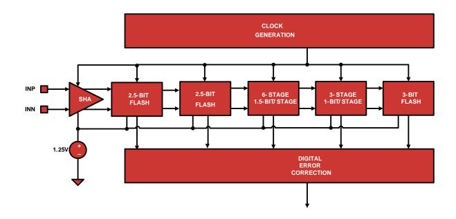
FIGURE 34. ADC CORE BLOCK DIAGRAM
