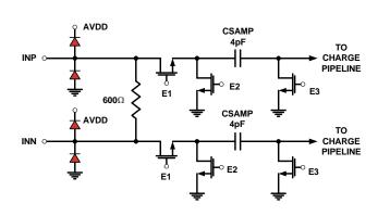
FIGURE 58. ANALOG INPUTS
