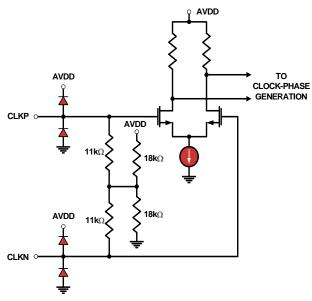
FIGURE 59. CLOCK INPUTS
