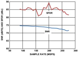
FIGURE 7. SNR AND SFDR vs f<sub>SAMPLE</sub>
