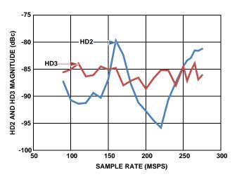
FIGURE 8. HD2 AND HD3 vs f<sub>SAMPLE</sub>
