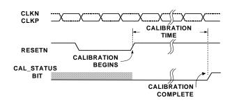
FIGURE 35. CALIBRATION TIMING
