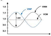
FIGURE 42. ANALOG INPUT RANGE
