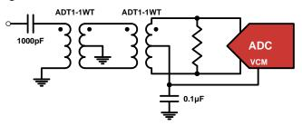
FIGURE 43. TRANSFORMER INPUT FOR GENERAL PURPOSE APPLICATIONS
