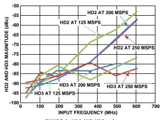
FIGURE 4. HD2 AND HD3 vs f<sub>IN</sub>
