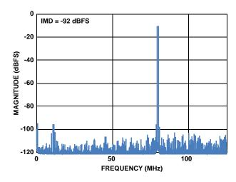
FIGURE 24. TWO-TONE SPECTRUM (F1 = 170MHz, F2 = 171MHz AT - 7dBFS) (250MSPS)
