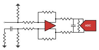
FIGURE 45. DIFFERENTIAL AMPLIFIER INPUT
