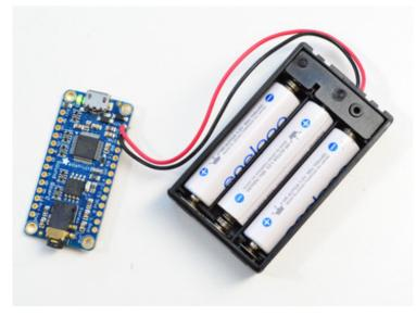
The nicer battery packs have switches, or you can just remove the batteries when not in use. If the green light is lit, it's powered up!
