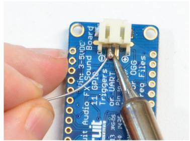
Solder all four pads - two mechanicals on the side, and two power coming out the end.
