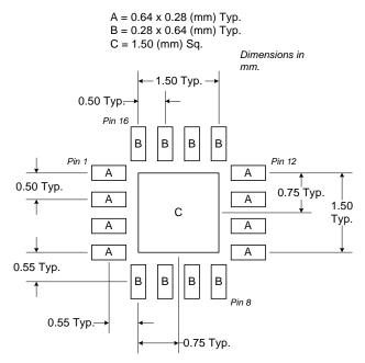
Figure 1. PCB Metal Land Pattern (Top View)
