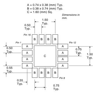
Figure 2. PCB Solder Mask Pattern (Top View)
