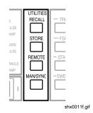
The **MAN/SYNC** key is used for manual triggering and synchronizing two or more generators when suitably connected together. Further information on synchronizing two generators is given in the *Users Manual*.
