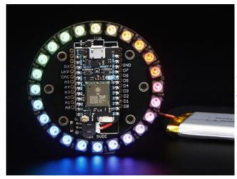
Previously mentioned on the "Rings" page, but for posterity: this <u>24-pixel</u> <u>RGB ring (http://adafru.it/2268)</u> is specifically designed for the Particle (formerly Spark) **Photon** development board.
