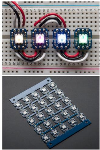
These are similar to the sewable Flora NeoPixels, but with a pin arrangement that (with the addition of headers) fits neatly into a breadboard for prototyping. Also available in two formats:
