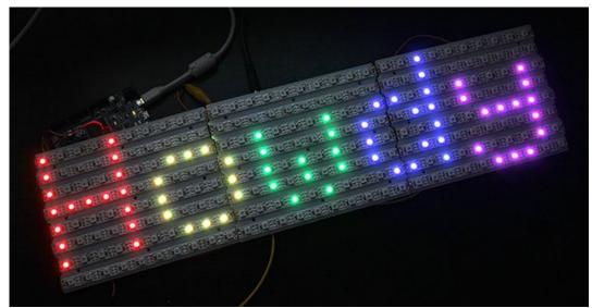
The Adafruit\_NeoMatrix library builds upon Adafruit\_NeoPixel to create two-dimensional graphic displays using NeoPixels. You can then easily draw shapes, text and animation without having to calculate every X/Y pixel position. Small NeoPixel matrices are available in the shop. Larger displays can be formed using sections of NeoPixel strip, as shown in the photo above.
