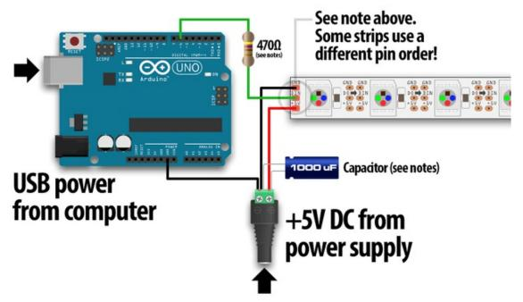
When connecting NeoPixels to any LIVE power source or microcontroller, ALWAYS CONNECT GROUND (–) BEFORE ANYTHING ELSE. Conversely, disconnect ground last when separating. When using a DC power supply, or an especially large battery, we recommend adding a large capacitor (1000  $\mu$ F, 6.3V or higher) across the + and – terminals. This prevents the initial onrush of current from damaging the pixels. See the photo on the next page for an example.
