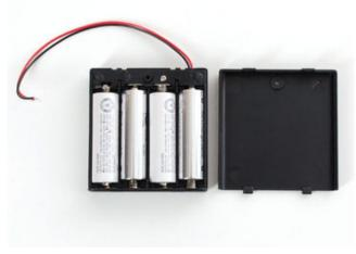
Four nickel-metal hydride (NiMH) rechargeable cells can similarly be used in a <u>4-cell battery</u> holder (http://adafru.it/830) to provide 4.8 Volts.
