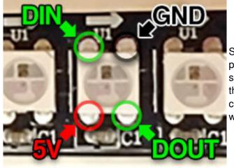
Some batches of 144 pixel strip don't have pads between the LEDs. If you cut these into shorter sections, the only way to connect to them (except at the half-meter segments) is to carefully solder directly to the LED. The corner with the notch is the GND pin.
