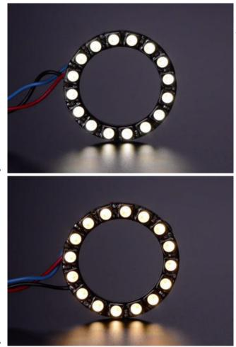
RGBW pixels incorporate a translucent **diffuser** layer to help mix and soften the light output. This makes them appear less intense than RGB pixels (which are "water clear"), but it's really the same LEDs inside.
