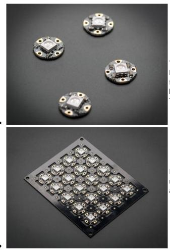
The original Adafruit NeoPixel form factor! **Flora RGB Smart NeoPixels** were designed for wearable projects using conductive thread, but can also be soldered normally with wires. These are available in two formats:
