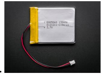
For many wearable projects we recommend a <u>lithium-polymer battery</u> (http://adafru.it/328). These deliver 3.7 Volts — perfect for directly feeding low-power microcontrollers such as the Adafruit Flora, yet enough voltage to run a short length of NeoPixels.
