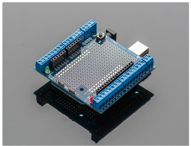
The shield even comes with <u>stacking headers</u>, (http://adafru.it/alH) which let you plug *another* shield on top! As shown here, a data logging shield is stacked onto the protoscrewshield.
