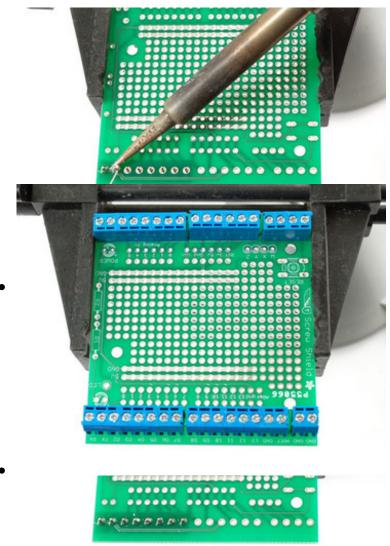
Place the remaining terminal blocks, checking again that they face the right direction!
