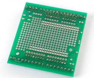
Solder all the pins of the header with plenty of solder.
