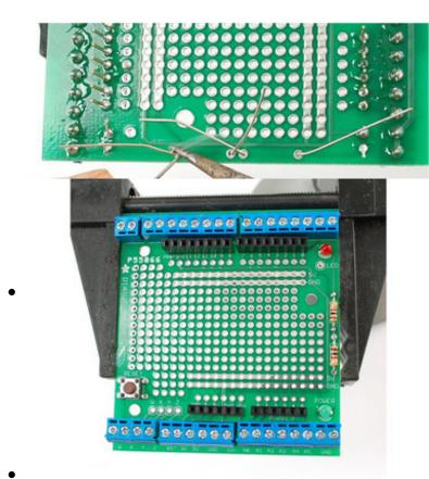
Last we will place the reset switch. This switch will let you easily reset the Arduino.
