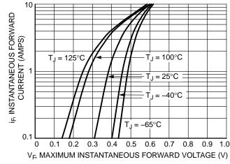
Figure 2. Maximum Forward Voltage
