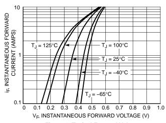
Figure 1. Typical Forward Voltage
