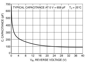
Figure 7. Typical Capacitance
