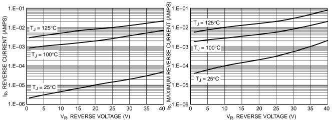
**Figure 3. Typical Reverse Current**
