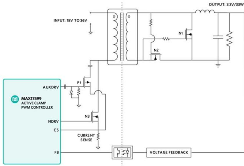
Figure 1. The MAXREFDES121# reference design block diagram.
