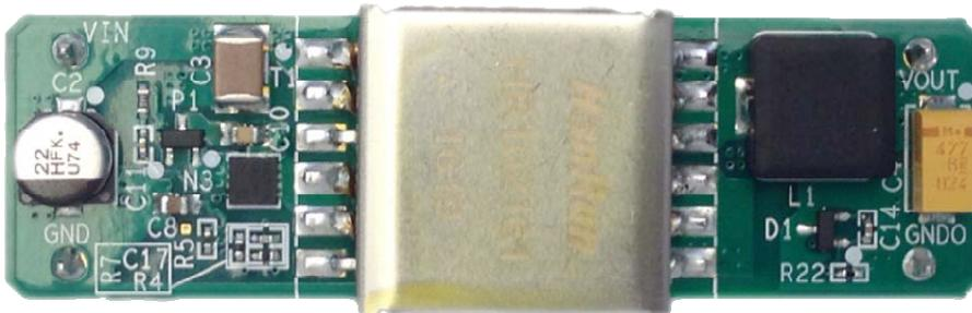
Maxim's power-supply experts have designed and built a series of isolated, industrial power-supply reference designs. Each of these power supplies efficiently converts 24V into useful voltage rails at a variety of power levels. Every power rail is isolated with a readily available transformer, providing quick, convenient transformer selection. Each design has been tested for load and line regulation, as well as efficiency and transient performance.
