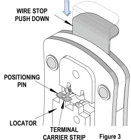
**Note**: The tamper proof ratchet action will not release the tool until it has been fully closed.
