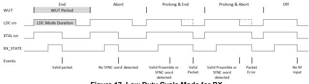
Figure 17. Low Duty Cycle Mode for RX
