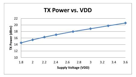
Figure 11. +20 dBm TX Power vs. VDD
