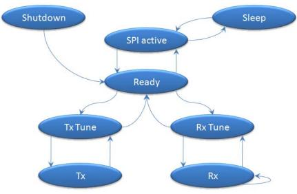
Figure 6. State Machine Diagram
