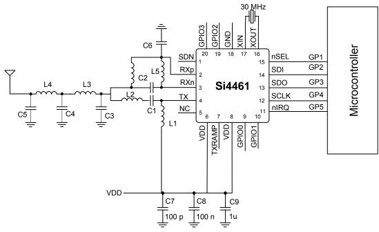
Figure 1. Si4461 Direct-Tie Application Example
