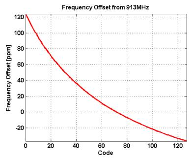
Figure 13. Capacitor Bank Frequency Offset Characteristics
