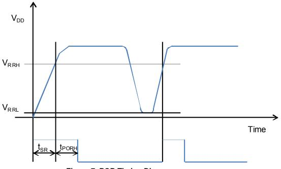
Figure 7. POR Timing Diagram
