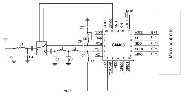
Figure 2. Si4463 Single Antenna with RF Switch Example
