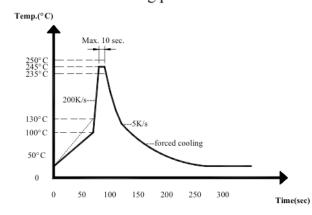
Recommendable wave soldering condition is as follows:
