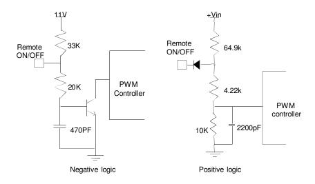
Figure 22 Remote ON/OFF internal diagram
