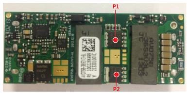
Figure 12 Temperature test point
