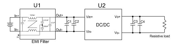
Figure 27 EMC test configuration
