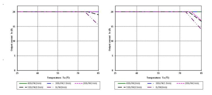
Figure 13 Output power derating,  $24V_{in}$ ,
