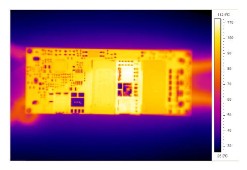
Figure 15 Thermal image,  $36V_{in}$ ,  $3.3V_{o}$ , full load, room temperature, 100LFM (air flowing from pin 3 to pin 1)
