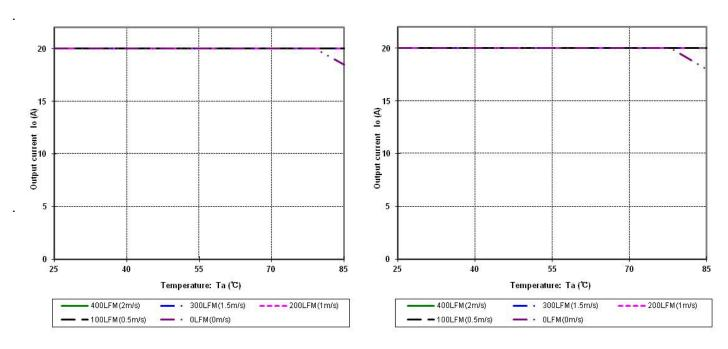
Figure 18 Output power derating,  $24V_{in}$ ,
