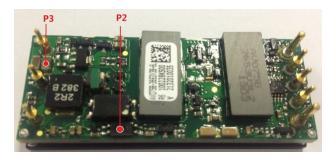
Figure 16 Temperature test point
