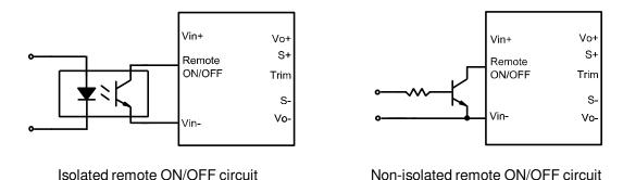
Figure 23 External Remote ON/OFF circuit
