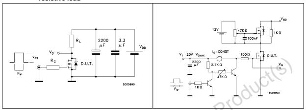
Figure 14. Test circuit for inductive load switching and diode recovery times
