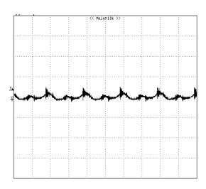
Figure 14: Output voltage ripple at nominal input voltage and rated load current (lo=40A)(20 mV/div, 2us/div)
