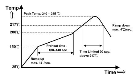
Note: The temperature refers to the pin of E48SH, measured on the pin +Vout joint.
