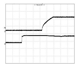
**Figure 7:** Turn-on transient at full rated load current (constant current load) (2 ms/div). Vin=48V.Top Trace: Vout, 1V/div; Bottom Trace: input voltage, 50V/div
