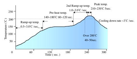
Note: The temperature refers to the pin of E48SH, measured on the pin +Vout joint.
