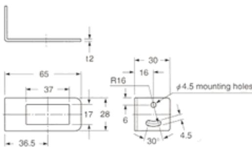
Material: Cold rolled carbon steel (SPCC)
