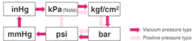
Note: 'MPa' when combining with DPH-A02, DPH-A12 or DPH-A22 positive pressure sensor head.
