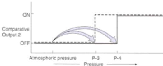
When there is no auto-reference input, the atmospheric pressure is taken as the reference pressure for Set Value P-3 and Set Value P-4.
