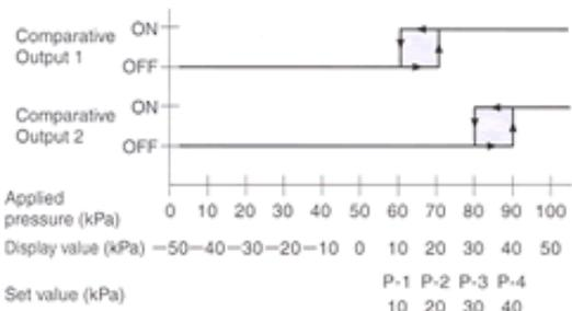
Note: In the hysteresis mode the displayed values and the ON/OFF points of the output are changed in case the output mode is set to the window comparator mode.
