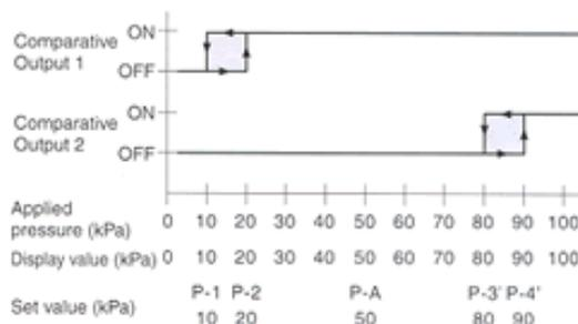
Note: In the hysteresis mode, Set Value P-3 and Set Value P-4 are shifted. The output is set to the window comparator mode or the leak test mode.
