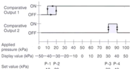
Note: In the leak test mode, the zero-adjustment function is applied only to Comparative Output 2. Comparative Output 1 operates with the atmospheric pressure as the reference.
