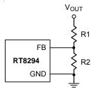
Figure 1. Output Voltage Setting
