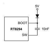
Figure 2. External Bootstrap Diode
