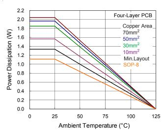
Figure 7. Derating Curves for RT8294 Package
