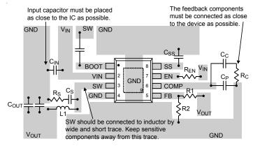
Figure 8. PCB Layout Guide
