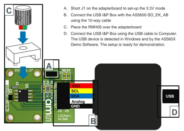
**Note:** It might be necessary to perform a firmware update on the USB I&P Box if a wrong firmware was detected. In this case, the user will be prompted to allow an automatic firmware upgrade.
