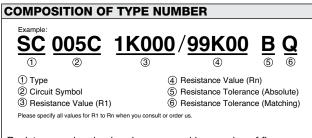
Resistance value, in ohm, is expressed by a series of five characters, four of which represent significant digits. R or K is a dual-purpose letter that designates both the value range (R for ohmic; K for kilo-ohm) and the location of decimal point.
