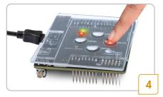
• Press BTN1 with the water on the overlay to evaluate CapSense water tolerance
