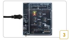
Place water droplets onto CapSense<sup>®</sup> buttons using the dropper provided
