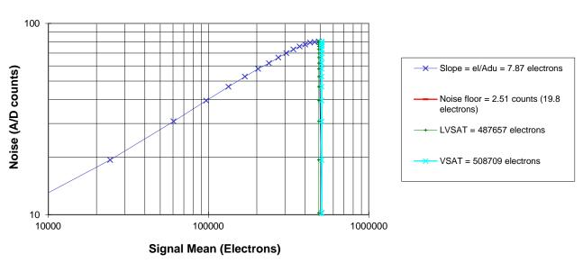
Figure 3. Measured Performance – Dynamic Range and Noise Floor
