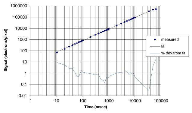
Figure 2. Measured Performance – Linearity
