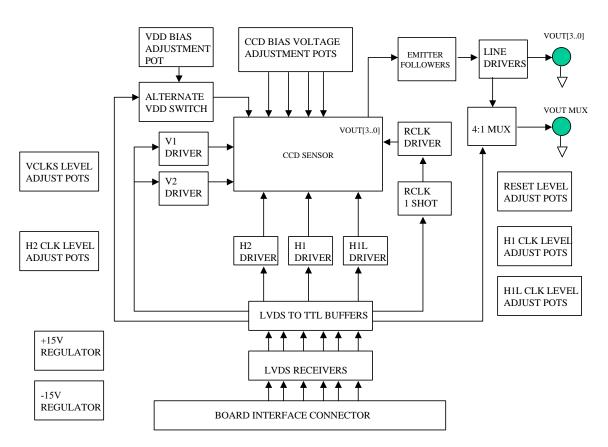
Figure 1. KAF-4320 Imager Board Block Diagram
